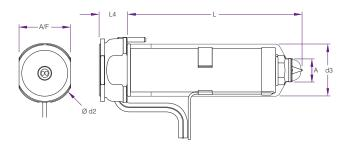
Low moulding temperature and pressure, excellent temperature consistency and front loading capabilities, that's the Mastip MX nozzle, specifically designed for multi cavity manifold systems and hot halves. The MX nozzle is suited for small to medium applications in all types of markets. It is able to process a wide range of plastics, from the easy ethylenes to tough engineering resins.
