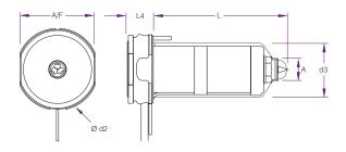
BX nozzle is designed to provide a cost sensitive solution to single & multicavity applications.
