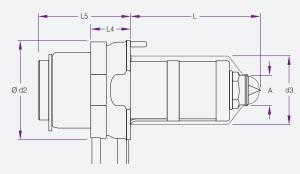
With two heaters the SX nozzle is perfectly suited for all single nozzle applications. Independently controlled heater zones provide uniform temperature distribution along the length of the nozzle, making it ideal to process difficult plastics.
