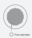
Used for Plastic Injection Moulding Pore Diameter: 0.03 ~ 0.10mm
