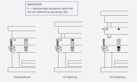
Mat.: 1.8159 Hardened 45 ± 3HRC Patented System No pocket machining required as needed with other similar products on the market. Minimum space required for installation. Reduces costs compared to conventional mechanisms. Offers a standard solution to the moulder.
